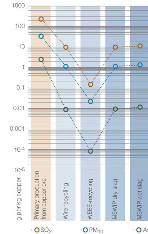
Fig. 7 Mass-related emissions of primary (brown bars) and secondary (blue bars) copper production. SO 2 : Sulphur dioxide, PM10: Particles ≤ 10 µm, As: Arsenic (10). Primary production creates significantly higher emissions.
